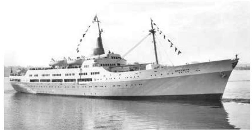
The Braemar with her combined signal mast and funnel. Photo from the Newall-Dunn collection. Reproduced from Anthony Cooke's book
