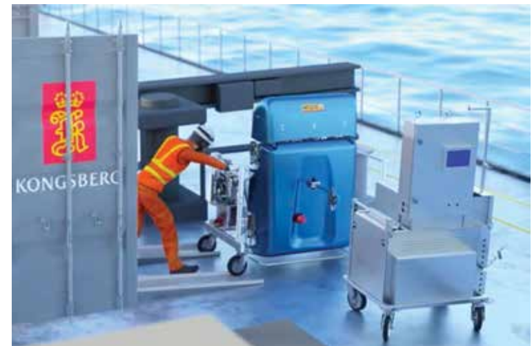
The hull skater being wheeled out ready for launching over the side. The image gives some idea of the size.
